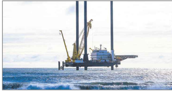
A liftboat vessel, an offshore workspace for South Fork Wind, New York's first offshore wind farm, in Wainscott.
